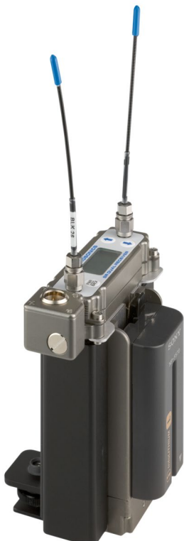
The receiver provides stand-alone operation with the battery sled adapter and mounting sleeve. It can be mounted in any position with Velcro, or in horizontal and vertical positions using the mounting foot, or mounted directly onto a 1/4-20 threaded stud on a tripod.
