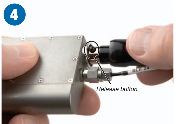
To remove the connector, pull the sleeve back to expose the black release button. Press the button to unlatch the plug.
