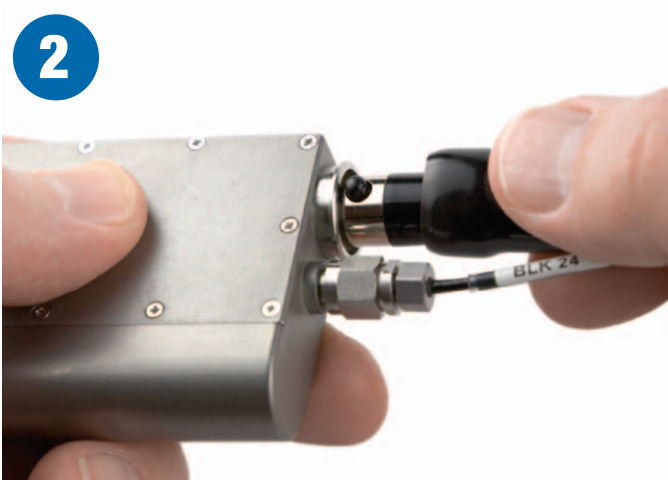
With the sleeve pulled back slightly, align the connector with the socket and insert until it latches securely.
