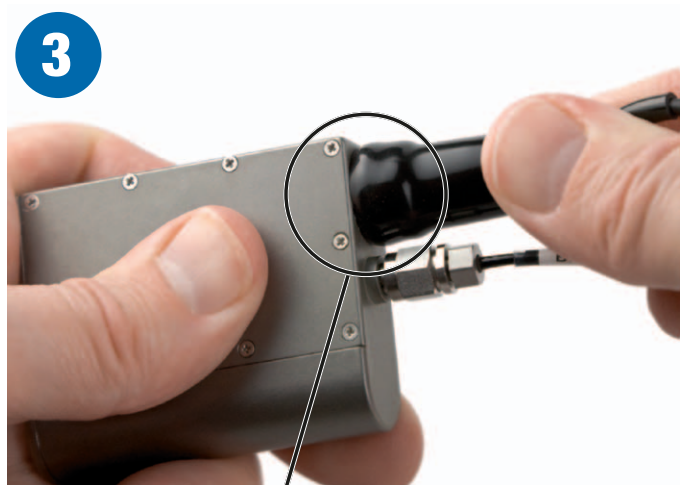
Slide the sleeve over the connector. Pinch and squeeze the sleeve near the flange and work it down with a kneading motion over the flange all the way around until it stays in place flush with the housing. Pull on the connector to make sure it is firmly latched.
