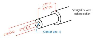
Mating power plug dimensions. P/N 21425 has a straight back shell. P/N 21586 has a locking collar.
