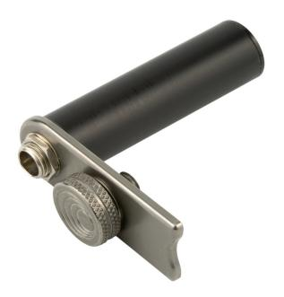
The SMBATELIM provides regulated 1.8 volts DC up to 1 amp to power all SM Series transmitter models for extended or continuous operation. The assembly is mounted to the transmitter housing in the same manner as the standard battery door. Circuitry is contained in a cylindrical housing in place of an AA battery, with a locking power connector.
