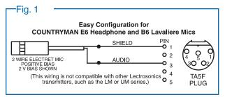
To set the bias voltage at 4V, install a jumper between Pins 2 and 4.
