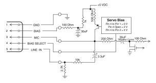
Lectrosonics Transmitter Equivalent Circuit
