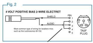
Install jumper between Pins 2 and 4 to set 4V bias. With no jumper, bias will be 2V.
