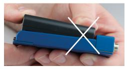
DO NOT insert battery contacts before pressing battery into the adapter.
