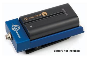
This handy accessory provides extended operating time and serves as a backup power supply for Lectrosonics transmitters and receivers. Common "L" and "M" style video camera rechargeable batteries are retained by spring tabs in the bottom plate. 9 volt batteries can also be used with the optional SR9VBP adapter.
