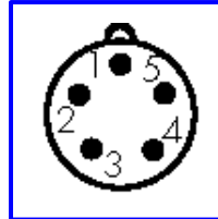
Figure 10-5 LEMO-5M Timecode Connector Pin Numbering
