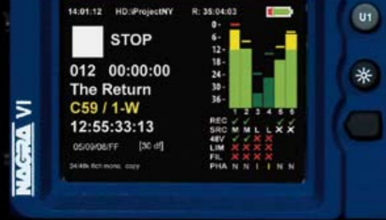
Main display screen: shows status, levels and menus of the recorder
